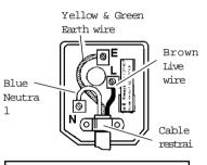
FUSE RATING THIS PRODUCT MUST BE FITTED WITH A 3 AMP FUSE
