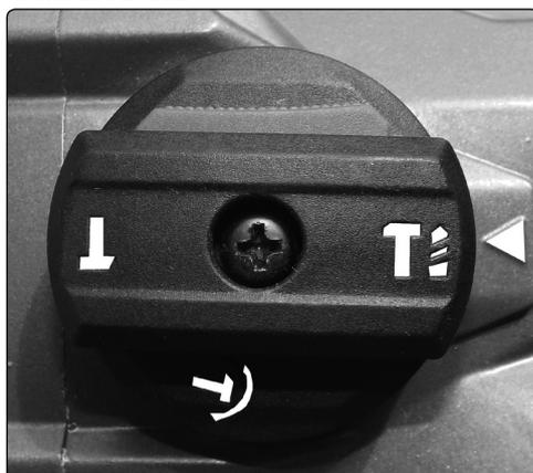
**NOTE:** It is not possible to operate the hammer drill with the hammer stop and rotation stop facilities both active at the same time.
