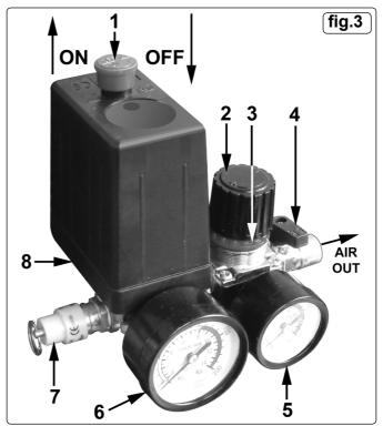
b) The main gauge (fig.3.6) indicates the pressure inside the main tank, **NOT** the pressure supplied to the air equipment, which is shown on the smaller gauge (fig.3.5). Should the pressure in the main tank exceed the pre-set switch (fig.3.8) maximum, the safety valve (fig.3.7) will activate. **WARNING!** For this reason **DO NOT** tamper with, or
