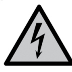
Electrical shock hazard
