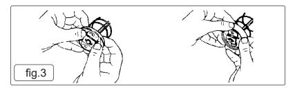
5.1.10. Put follower back into barrel, tighten the barrel cap & follower assembly with the barrel.
