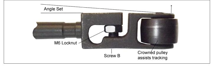
Method:- From this position shown, loosen the locknut by 2 full turns. Then, as in 5.1.5., replace the belt, reconnect the air supply and operate the sander, observing the tracking of the belt. Adjust the tracking by turning the screw 'B' clockwise, changing the "Angle Set" until the belt is running true. When the belt is running true, switch off, disconnect from the air supply and remove the belt, as in 5.1.3. Secure screw 'B' into position with the locknut and replace the belt.
