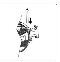
Align hose reel assembly with the holes in the bracket. Insert the pivot bar through the bracket and reel. Connect short hose on back of reel to water supply.
