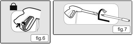
6.1.8. Unlock the lever on the pressure gun.
