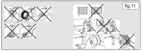
6.3.1. Use the pressure washer only if the hose is completely uncoiled and extended. See fig.11.
