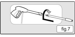
6.1.8. Unlock the lever on the pressure gun.
