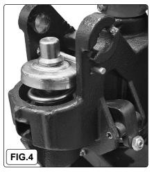
Keep the pin in position until AFTER assembling the handle.
