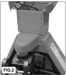
Attach the display housing with the fixings supplied.
