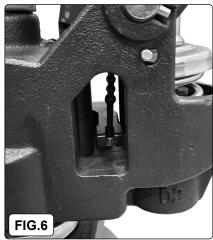
Attach the release rod chain to the adjusting nut.
