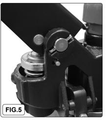
Secure the handle using the handle axle and spring pins.
