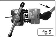
4.7. Pull the lever to engage the punch into the end of the brake pipe and continue to form the flare until a solid resistance is felt (Fig.5). Return the handle to the original position to withdraw the punch. If the required flare calls for a second operation in Chart 1, slide the correct Op.2 punch in line with the brake pipe. Operate the lever to complete the form of the flare.
