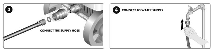
4.2 Connecting the water supply. Screw the hose connector to the water inlet on the machine (see fig.3). Use a reinforced hose pipe with an internal diameter of 1/2" and connect to the mains water supply as indicated in fig.4.
