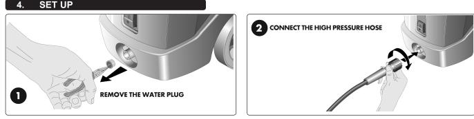
4.1 Connecting the high pressure hose. Remove and discard the transit plug from the water 'out' connector on the lower front of the machine (see fig.1). Attach the high pressure hose as indicated in fig.2 ensuring that the connector is tight.
