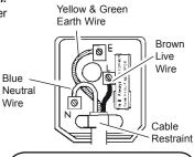
**FUSE RATING** THIS PRODUCT MUST BE FITTED WITH A 13 AMP FUSE
