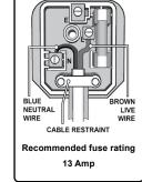
C) After wiring, check that there are no bare wires and ensure that all wires have been correctly connected.
