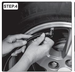
4. Connect the air hose to the tyre valve stem. Ensure the connector is secure.
