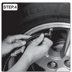
4. Connect the air hose to the tyre valve stem. Ensure the connector is secure.
