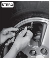
3 Connect the air hose to the tyre valve stem. Ensure the connector is secure.
