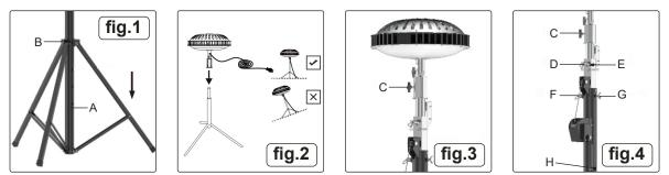
4.4.1. Fold out the legs to the desired length from the center tube (A). Stand the tripod on its feet (taking account of any unevenness in the terrain, if applicable) see fig.2. The bracket contains multiple adjustable holes to compensate for differences in ground height. It is essential that the stand is levelled before loading with equipment. Secure wing nuts (B) on the tripod see fig.1. Note: If you DO NOT tighten the wing nuts the telescopic tube may retract under load.
