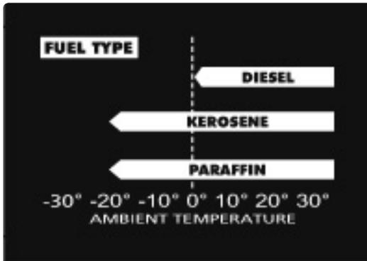
Although this heater operates with diesel fuel, when the temperatures are below 0°C, diesel additives are required to maintain the diesel's viscosity. Typically diesel can cloud in freezing conditions and will start to gel. You will need additives for your fuel in these conditions. Kerosene/Paraffin does not start to gel until the ambient temperature is around -40°C.
