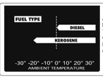
Although our heaters operate with diesel fuel, when the temperatures are below  $0\,^{\circ}\text{C}$ , diesel additives are required to maintain the diesel's viscosity. Typically diesel can cloud in freezing conditions and will start to gel. You will need additives for your fuel in these conditions.
