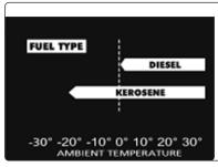
Athough our heaters operate with diesel fuel, when the temperatures are below  $0^{\circ}$ C, diesel additives are required to maintain the diesel's viscosity. Typically diesel can cloud in freezing conditions and will start to gel. You will need additives for your fuel in these conditions.
