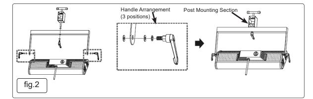
4.1.1. Assemble lamp arrangement using the adjustment handle, spring washer and plain washers (fig.2) in two positions shown.
