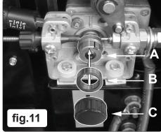
**5.5. SETTING WIRE TENSION**. Adjust the wire tension by rotating the wire tension control. Turn clockwise to increase the tension and anticlockwise to decrease the tension. See fig 10.1.
