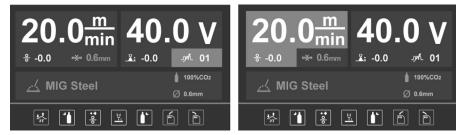
i: Basic parameter settings are: gas pre flow, slow wire feeding, gas post flow, operating, load and save function.
