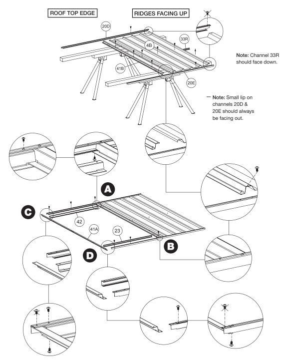
Fit part 41A (jamb), part 42 (jamb) and part 23 (bottom channel) and fix them with the self tapping screws (except those marked with a cross). Make sure both joins (diagrams A and B) are fixed the same followed by diagrams C and D.
