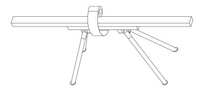
Place 2 x part 6A (sheet) on your worktable and join together with the self-tapping screws as per the diagram below.
