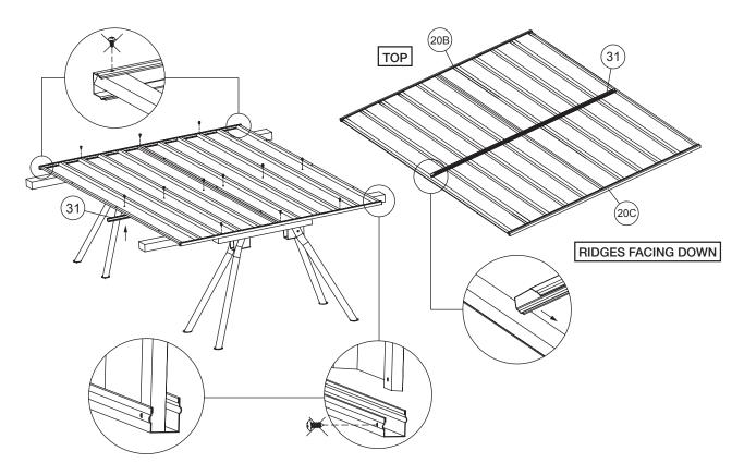
Tip: If panel and screw holes do not line up, try pulling panel to match up holes.
