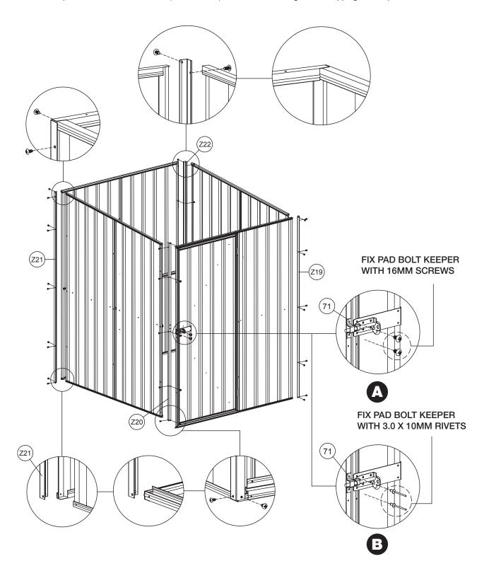
Now fit the bolt down kit as per the diagram. Strengthen the mid wall braces by applying part 72 (mid wall brace bracket) to each corner if necessary.
