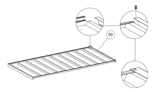
7.4.3 Fit item 50 (angles) to each edge, refer to diagram this page for flange orientation. Fix with 10mm long self tapping screws.
