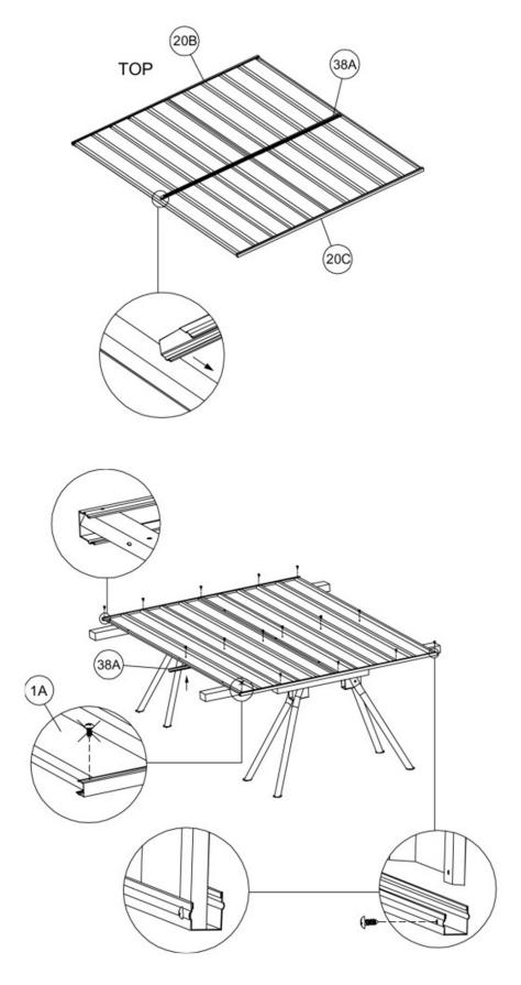
7.1.4 Fit item 38A the mid height wall channel to the panel and position it by the pre-punched holes and 10mm long self tapping screws. Note this channel is fitted with the flat face uppermost, ie. nearest the "top".
