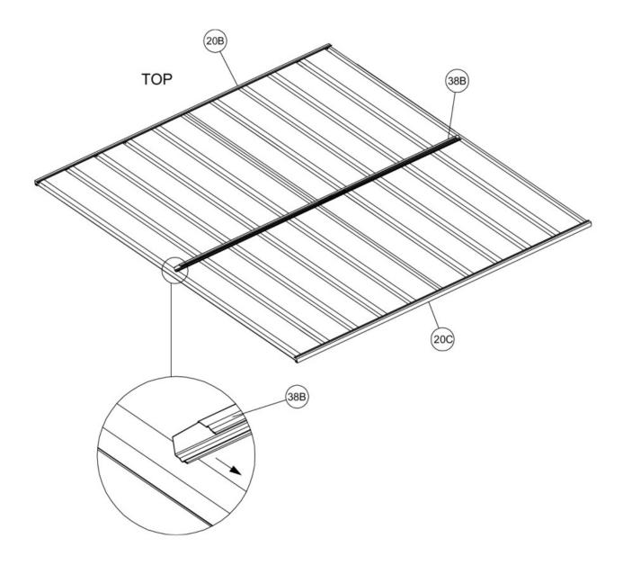
7.3.3 Fit item 38B the mid height wall channel to the panel and position it by the pre-punched holes and 10mm long self tapping screws. Note this channel is fitted with the flat face uppermost, ie. nearest the "top".
