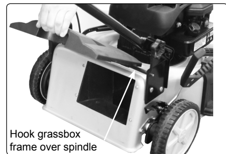
Hook grassbox frame over spindle Lift stone guard hinged panel to fit grass box.
