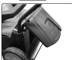
Lift spring loaded hinged stone guard panel to fit grassbox. (2 tabs along top of opening)
