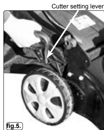
Adjust cutter height
