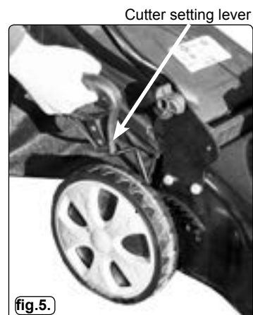
Adjust cutter height
