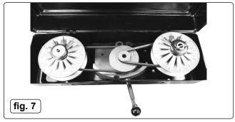
8.4.6. Run the drill to re-tension the belts.
