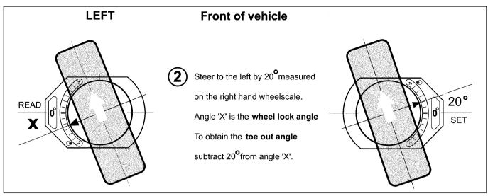
4.3 Measure the **WHEEL LOCK ANGLE** and the **TOE OUT ANGLE** for both left and right steering as described above and below. COMPARE YOUR READINGS WITH THE VEHICLE MANUFACTURERS RECOMMENDATIONS.
