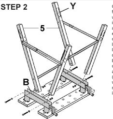
Open the leg frames (5) and align with holes on the inside of the vice arms at points "B" ensuring the curvatures on the lower part of the legs "Y" point outward. Insert bolts (3) from the outside of the vice arm with washers (7) and secure with washers (7) and nuts (11) from the inside
