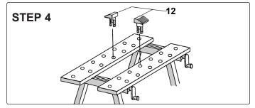
Fix chock (12) in suitable holes located in worktop as required.
