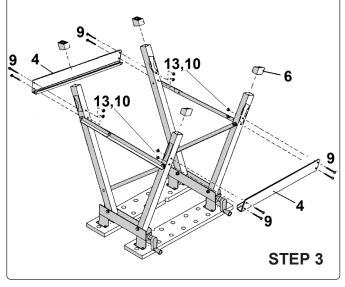
Align the crossbars (4) with holes in legs and insert screws (9) from the outside and fix with washers (13) and nuts (10). Push the plastic feet (6) onto the leg ends ensuring the longest side of the foot corresponds with the outer corner of the leg point.
