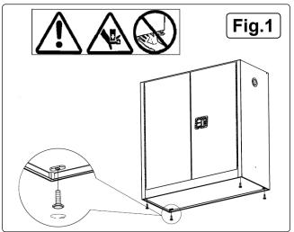
4.4.1. The cabinet comes with pre-installed levellers on the bottom of the unit. For best results ensure that the cabinet is level from side to side and has a slight tilt (2°) from front to back to prevent spillage, see below.
