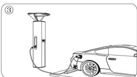
**DO NOT** disconnect the charging cable whilst the vehicle is charging
