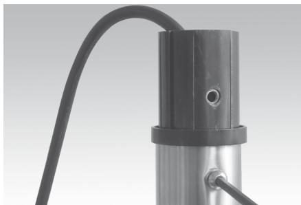
3.4 Fit a connecting tube into the base tube and secure with 3 x allan bolts.
