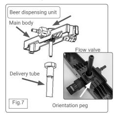
• Screw the delivery tube over the pick up tube on the underside of the assembly making sure that the 'O' ring seal is in situ and in good condition in the top of the delivery tube. Replace seal if in doubt.
