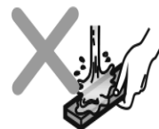
Washing is prohibited as it will damage the antibacterial properties of the filter
