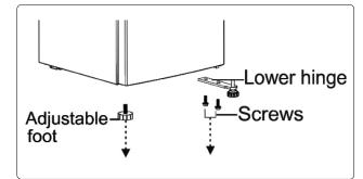
5. Remove the adjustable foot on the lower hinge shaft, and remove the washer and nut.
