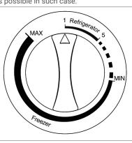
9. Estimate the number of food to be frozen. When freezing large amounts of fresh food, adjust the temperature control knob to the low mode, with the freezer temperature lowered. So, foods can be frozen up in a fast manner, with the food freshness retained.
