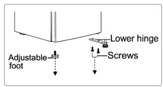
5. Remove the adjustable foot on the lower hinge shaft, and remove the washer and nut.
