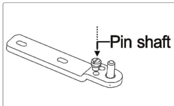
7. Install the lower hinge on the left side of the cabinet.
