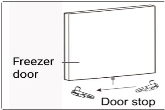
9. Installing the freezer compartment door.
