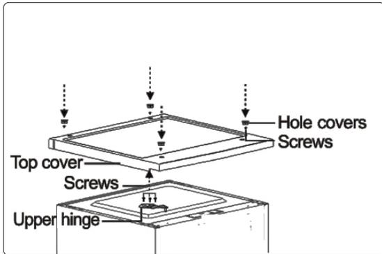
**NOTE:** When installing the door, ensure that the top of the door is level with the top of the cabinet. If the door is not level, the rubber gasket will not make a good seal which will cause the freezer to malfunction.
