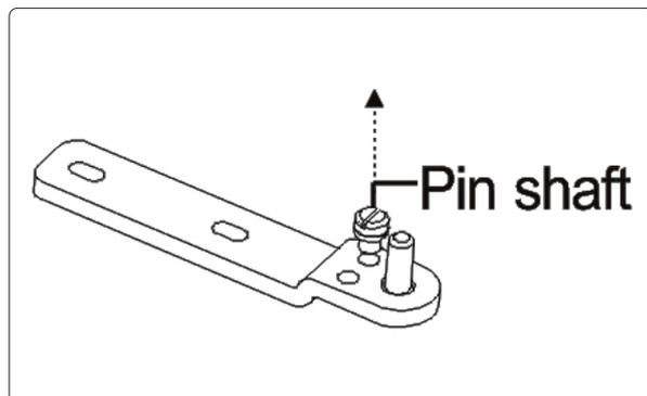
6. Insert the pin shaft into the left hole on the lower hinge, then secure the shaft with the washer and nut.
