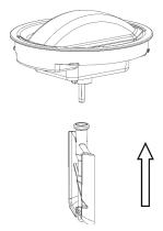
**Step 4.**Install the mixing fan blade.
