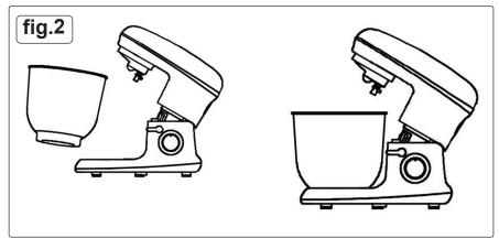
Place the mixing bowl (2) on the device plate, and turn the mixing bowl unit in clockwise direction until it is fixed, fig.2.
