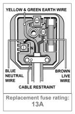
A) Connect the GREEN/YELLOW earth wire to the earth terminal 'E'. B) Connect the BROWN live wire to the live terminal 'L'.
