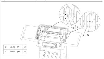
Step 6 Install the levelling bar attachments, ensuring they are firmly and correctly positioned.
