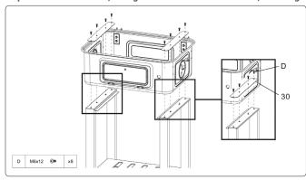
Step 3 Secure the BBQ body onto the base.
