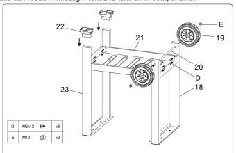
Step 1 Fit the legs and wheels into position on the grid-style base.
