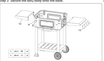
Step 5 Install hooks and fasten the side shelves securely.
