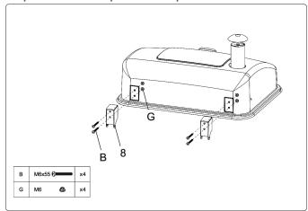
• Step 11 Secure hinges to the lid and align with the body.
