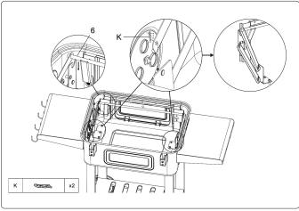
Step 7 Secure the riser bar in place.
