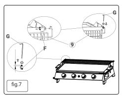
· Using screw fixings F and Allen key G (fig. 7).
