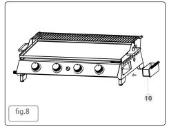
• Attach drip tray 10 to side of gas plancha
