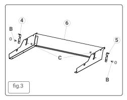
Attach brackets 4 & 5 to shield using screws B and washers and nuts C (fig. 3).
