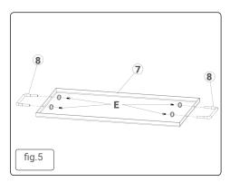
Attach carrying handles 8 to warming rack 7 using screws E (fig. 5).
