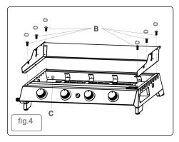
Attach shield 6 using screws B and washers and nuts C (fig. 4).
