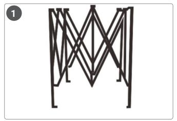
Place the gazebo on its feet in the centre of the area to be sheltered. Check to ensure that the roof struts are not stuck before moving.
