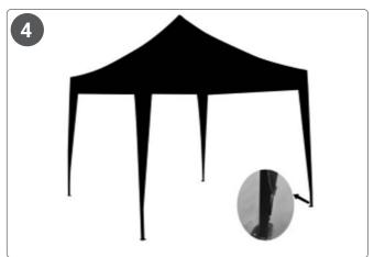
Raise or level the shelter using adjustment holes found near bottom of each outer leg. Secure with guide ropes/weight bags.
