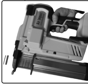
B. Loading nails:
