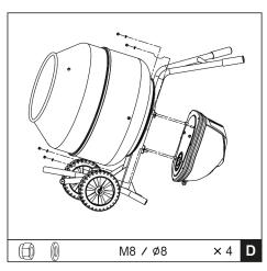
D: Lining up the keyways, slide the transmission case over the pinion shaft. Secure a nut with flat washer on each of the four stub bolts.
