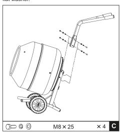
C: Lining up the holes in the handle bar with the ones in the support frame. Secure them together with bolts, lock washers and flat washers.
