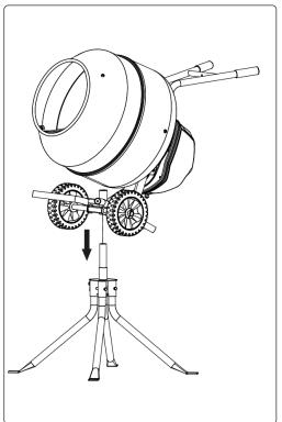
Place support stand into the whole in the axle bracket as shown.
