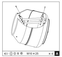
A: Insert the cross headed screws from the outside through the holes in the drum.
