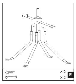
E: Insert the support legs into the bracket and secure them together with shaft and hairpin.
