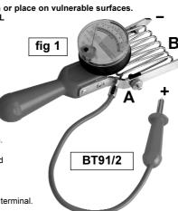
The meter reading, for a healthy battery, should be between 11.5 and 12.5 volts for a 12 volt battery or between 5.5 and 6.5 volts for a 6 volt battery.
